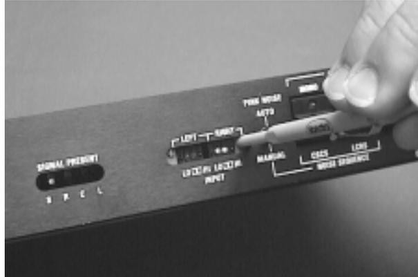
**Figure 4-2 Adjusting the Right Input Trim Control**
