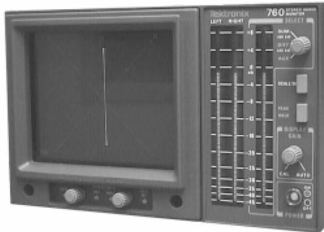
**Figure 2-21 Tektronix 760 Phase Scope Display of Center Channel Information**
